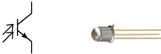
Fig. 7.8 : (a) symbole du phototransistor, (b) Phototransistors.
